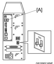
6. Turn the main power switch of the E-7000 to On and wait until installation is complete. Installation takes approximately 15-25 minutes. The LED on the flash drive should show that files are being transferred. The E-7000 shuts down automatically after installation is complete.
