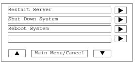
**NOTE:** Do not reboot the E-7000 by turning the copier main switch OFF and ON. Recycling power to the copier does not reboot the E-7000 properly.
